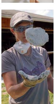
**Ball test.** Form a ball of plaster. It shouldn't fall apart when tossed, and should stick to the inside wall of a wheelbarrow when thrown against it.
